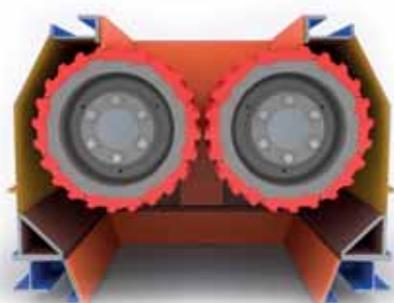
Cut through the crusher DVU for coarse crushing
