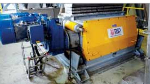
Crusher DVU 630x1500 – fertilizer crushing 25t/h
