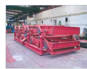
Resonant screen RT 2087/2 – in the manufacturing plant
