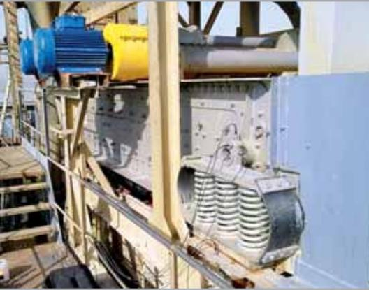
Screen EDT2N2160/2PU positioned on a pontoon – wet screening of gravel from the seabed
