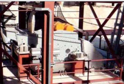
Screen EDT2N1430/2FeK – dosed screening of limestone to shaft kilns
