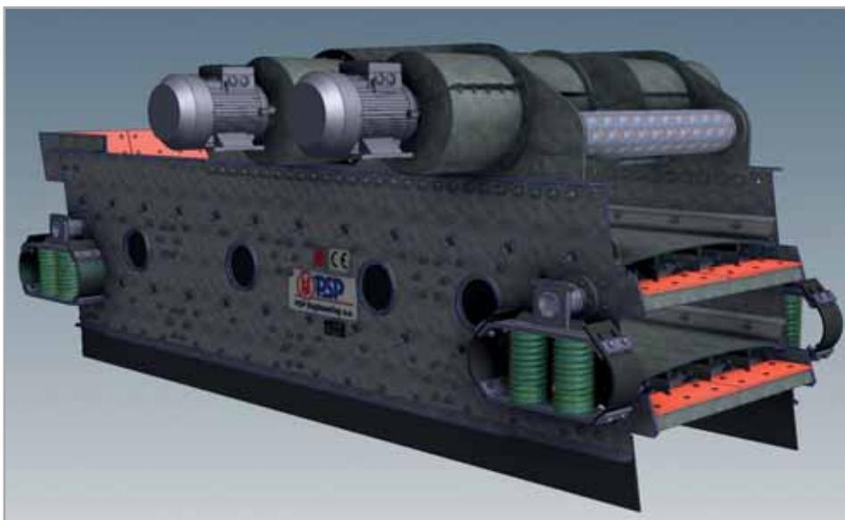
PC 3D model of the screen EDT2N1240/2Fe
