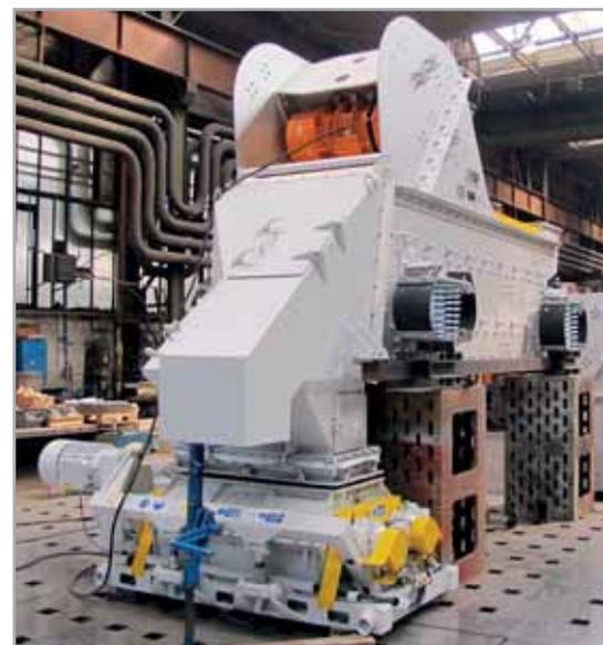
Final workshop assembly of the screen EDT2N1030/2Fe-150°C. Screening of slag of 150°C and subsequent finish-crushing in the crusher DVR.
