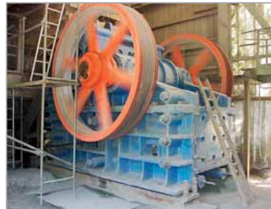
Jaw crusher V10-2N – gabbro crushing
