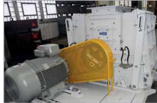
Crusher KMR 0808 in the manufacturing plant
