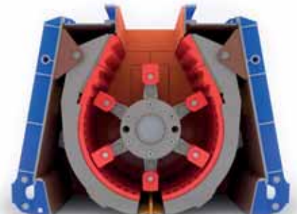
Mill KMR with grate plates
