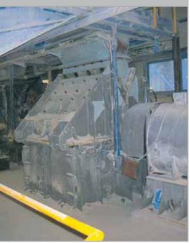
Hammer crusher KMR 2145 – crushing of limestone for desulphurization
