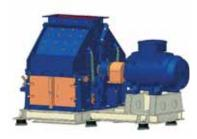
3D model of the hammer crusher KMR 2142 with the drive on the common anchoring frame
