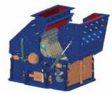
3D model of the hammer crusher KMR 2142
