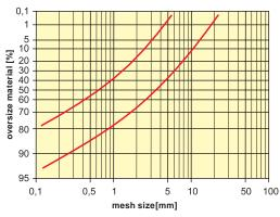
The field between curves characterizes the crushing ability of machines that depends on the inlet size, the slot of the grate and kind of material crushed.
