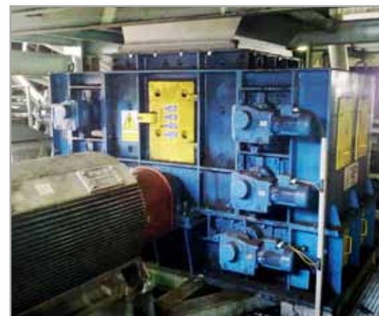
Crushers KDV 1313 – coal crushing 400t/h
