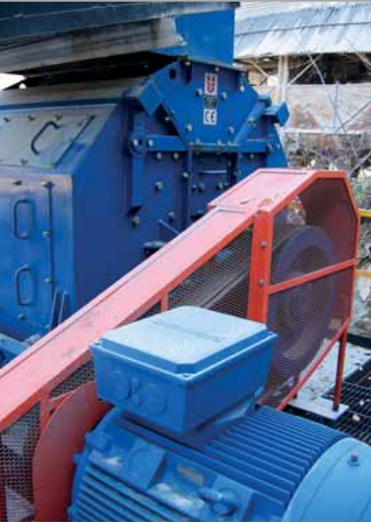
Crusher ODJ 1010-4 – limestone crushing 80t/h
