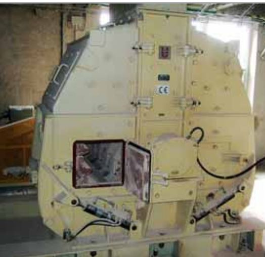
Crusher ODJ 1010-4 – limestone crushing 60t/h
