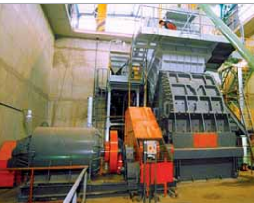
Crusher OKD 2020 – limestone crushing 450t/h
