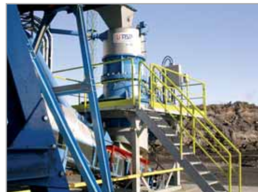
Cone crusher KDC 23 HP - slag crushing
