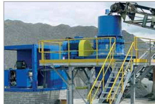
Cone crusher KDC 33 JP – spilite crushing
