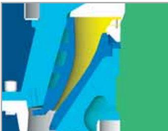
Crushing chamber of the tertiary crusher
