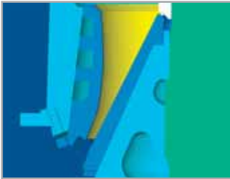
Crushing chamber of the secondary crusher
