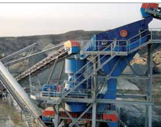
Cone crusher KDC 36 GP – basalt crushing
