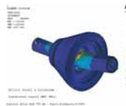
Computing analysis of a cone with the shaft for the cone crusher KDC. Stress in the solid model.
