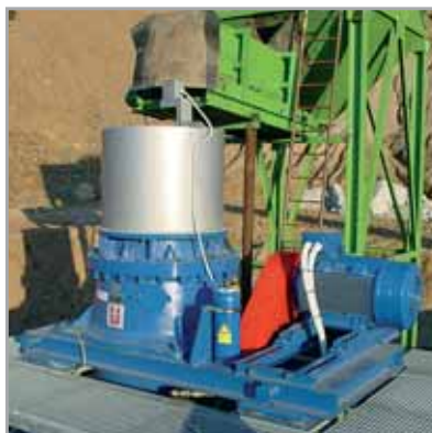
Cone crusher KDC 33 FP – granite crushing
