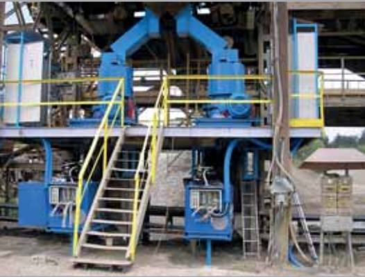
Cone crushers KDC 32 JP - gravel crushing
