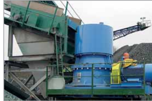
Cone crusher KDC 35 GP – andesite crushing
