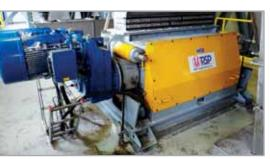
Crusher DVU 630x1500 – fertilizer crushing 25t/h
