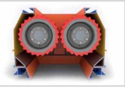
Cut through the crusher DVU for coarse crushing
