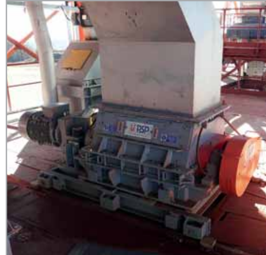
Crusher DVZ 30 - lime crushing 25t/h
