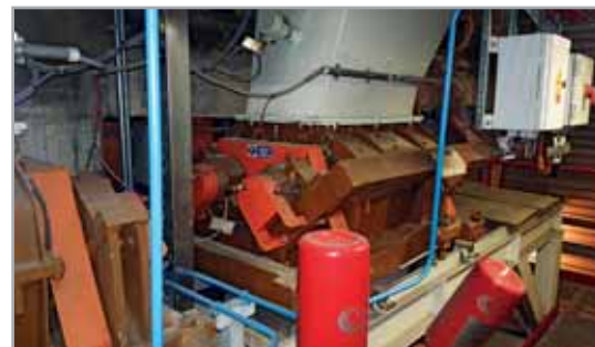
Crusher DVR 10 – coal crushing 10t/h
