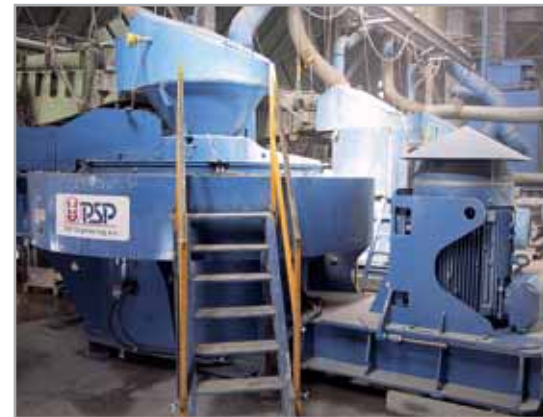
Crusher ODV 12SM – granite crushing 200t/h
