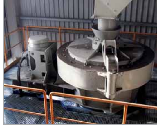
Crusher ODV 8SM – spilite crushing 70t/h
