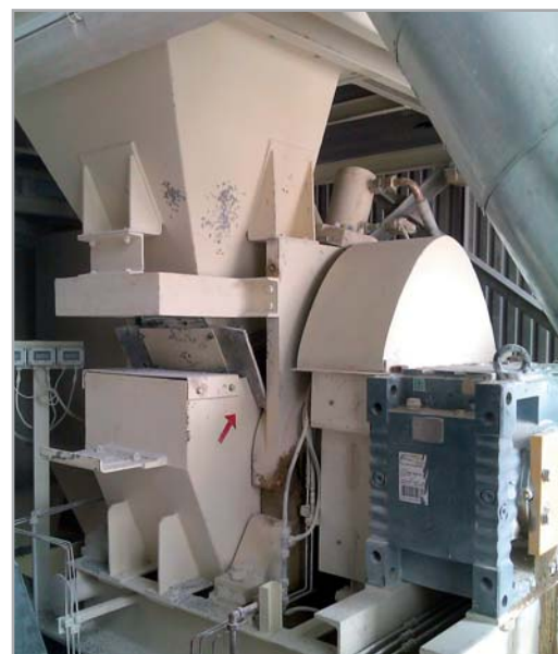
PREMILL PM 800 – limestone grinding
