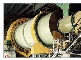
Raw mill Ø 5.4 x 11 m with a pre-drying chamber
