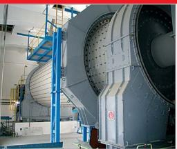
Cement grinding plant with a Ø 4.0 x 13.75 m mill seated on shoe-type bearings
