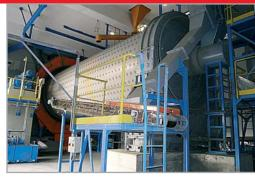
Cement grinding with a Ø 4.0 x 13.75 m mill seated on shoe-type bearings
