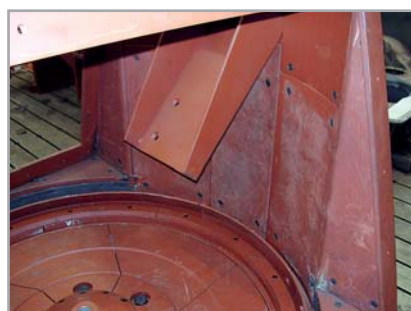
Grinding chamber armored with HARDON and cast segments of grinding table
