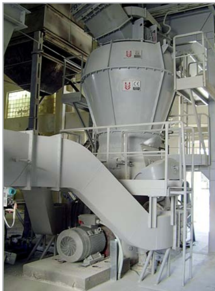
Lime grinding plant with KTM 1200
