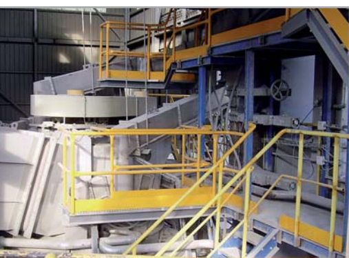
Mill separator DTIM 2500 with upper feeding of grist
