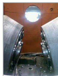
Hard faced grinding runners and grinding chamber lining
