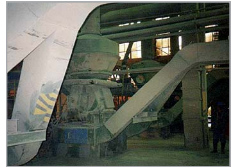
Existing mill KTM 1200 before disassembly and installation of a new mill on the existing foundation
