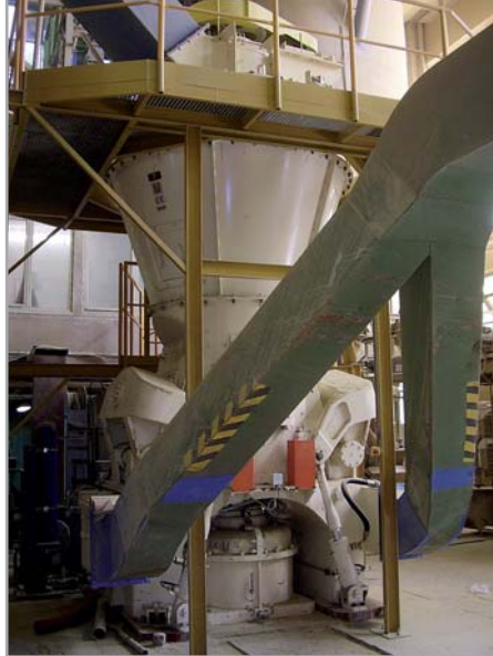
A new mill KTM 1200 installed on existing foundation frame of existing mill KTM in customer's plant - bentonite grinding.
