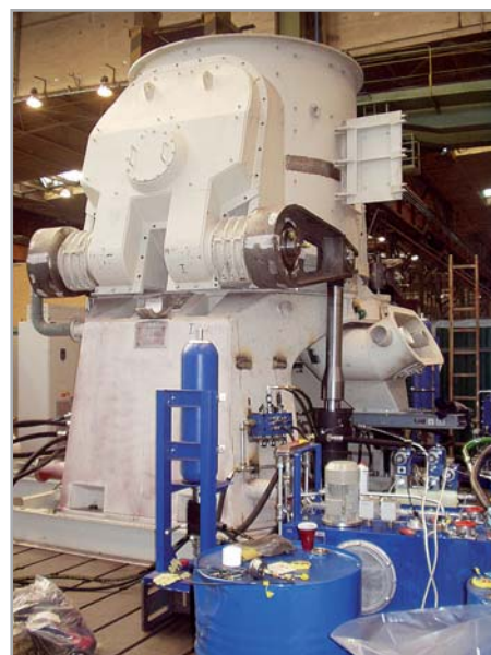
Assembly of a KTMU 1800 for grinding of coal in PSP's work shop
