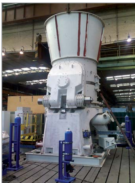
Assembly of a KTMU 1800 for grinding of coal in PSP's work shop
