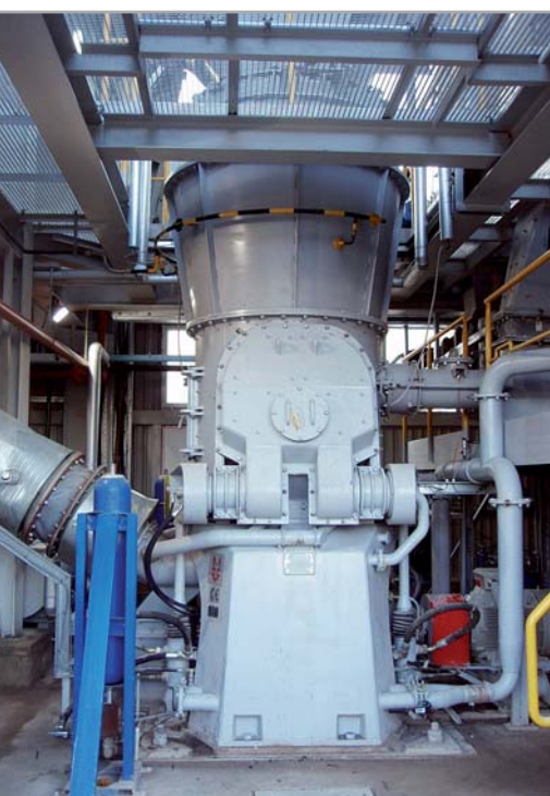
KTMU 1200 for grinding of petroleum coke and anthracite
