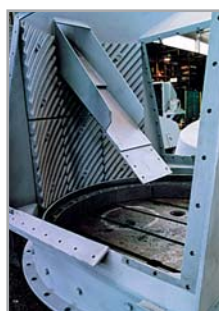
Cast lining of the grinding chamber
