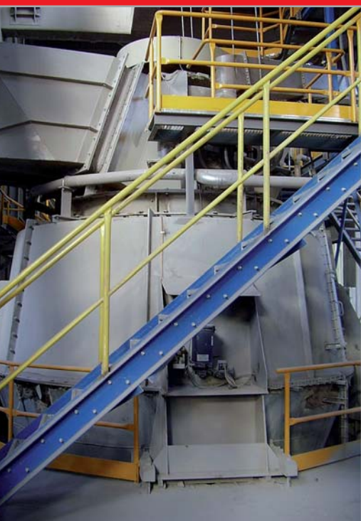
Mill separator DTIM 2500 with upper feeding of grist
