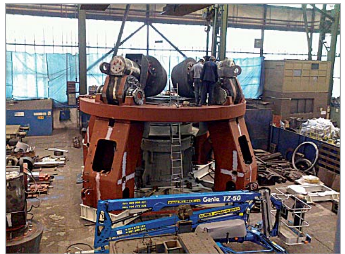
Placement of grinding carrier in the bearings
