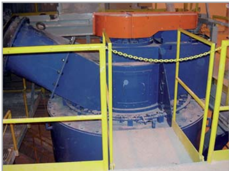
DTIM 1500 separator of a vertical mill installed on a KTM 1400
