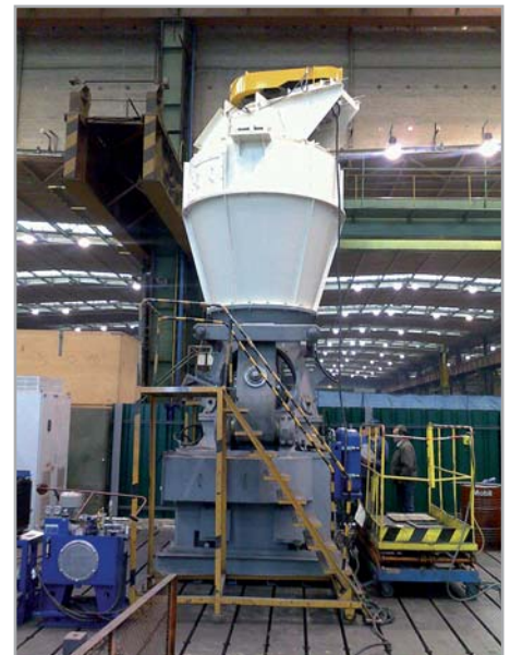
Reconstruction of a KTM 1200 in PSP's work shop
