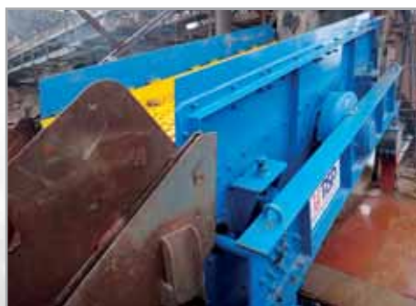
Operation with the coarse screen HT1540 – paragneiss screening 400t/h
