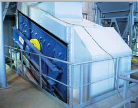
Installation of the coarse screen HT1540/2 – limestone screening
