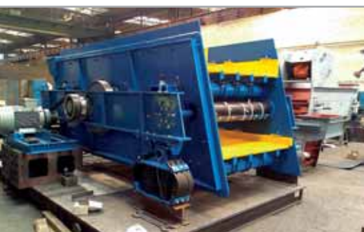
Manufacture and tuning of the coarse screen HT1540
