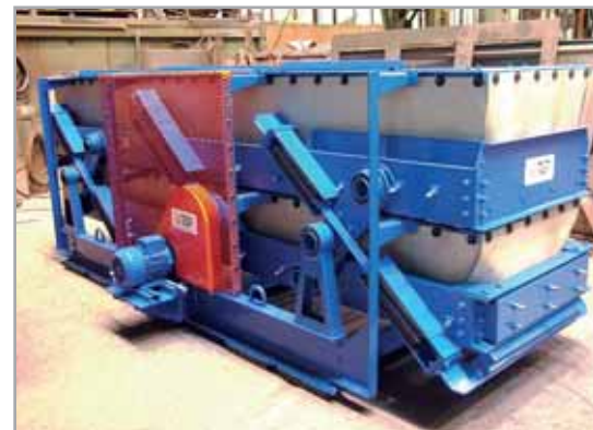
Manufacture of the resonant screen RT1047 – glass recycling
