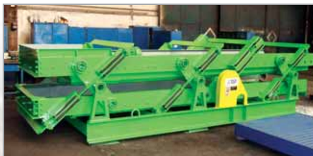
Manufacture of the resonant screen RT2057 – glass recycling
