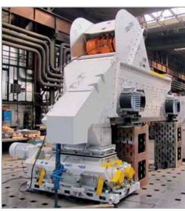
Final workshop assembly of the screen EDT2N1030/2Fe-150°C. Screening of slag of 150°C and subsequent finish-crushing in the crusher DVR.
