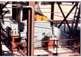
Screen EDT2N1430/2FeK – dosed screening of limestone to shaft kilns
