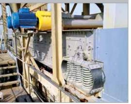
Screen EDT2N2160/2PU positioned on a pontoon – wet screening of gravel from the seabed
