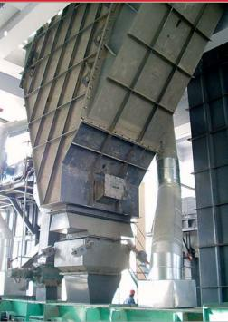
Above: Cascade air separator KVT 1800 as part of the 120 tph cement grinding plant at Qilianhan Cement, China. The photo shows the lower part of the separator with the coarse fraction discharge
