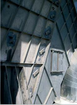
Above: View of the separator central section with manholes for easy access during maintenance
