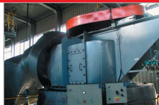
Air separator LTR-R 1650 at the coke grinding plant with 12.5 t/h capacity – OKD Ostrava, Czech Republic
