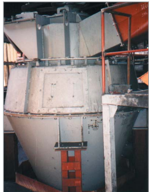
Air separator LTR-R 1250M at the TiO 2 slag grinding plant with a capacity of 4.5t/h – Celje, Slovenia
