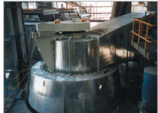
Air separator LTR-R 2500 at the cement raw material grinding plant with a capacity of 105t/h – Rezola, Arrigoriaga, Spain
