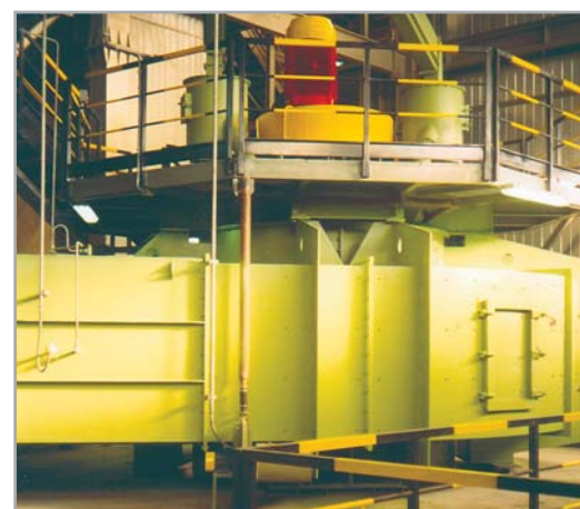
Air separator VTP 2900 at the cement grinding plant with a capacity of 130t/h – Galatina, Italy
