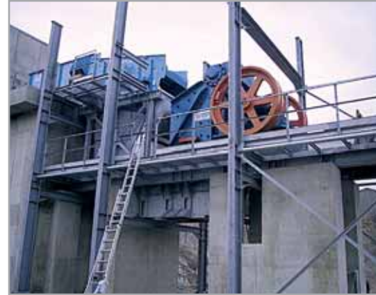
Jaw crusher DCD 4706 - granodiorite crushing
