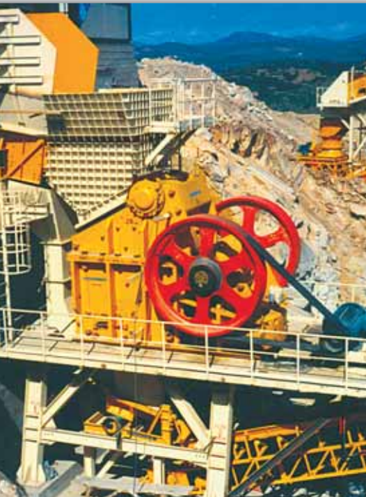
Jaw crusher DCD 4706 arranged in the treatment line for granite crushing
