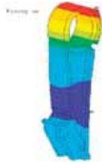
Computer analysis of the pendulum of jaw crusher. Displacements in the solid model.
