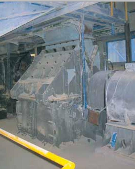
Hammer crusher KMR 2145 – crushing of limestone for desulphurization
