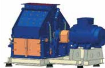
3D model of the hammer crusher KMR 2142 with the drive on the common anchoring frame
