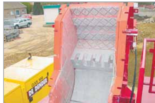
Opened housing of the impact crusher ODR 1051
