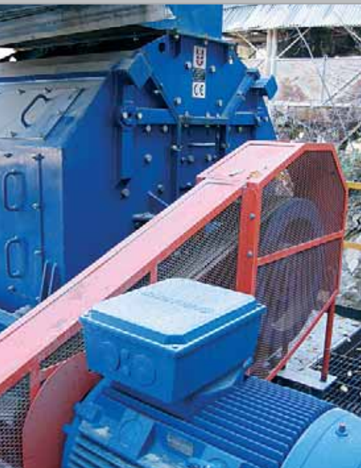
Impact crusher ODJ 1122 – limestone crushing
