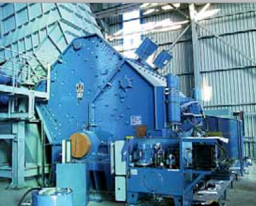
Impact crusher 1000t/h – cement material crushing
