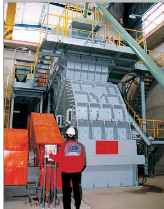
Impact hammer crusher OKD 1155 – cement material crushing
