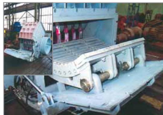
Impact hammer crusher OKD 1155 – tilted part of the housing with the grate
