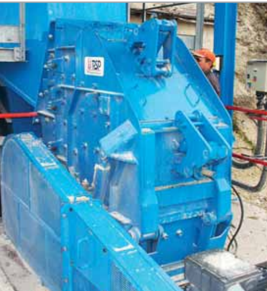
Crusher ODH 0907-12 – dolomite crushing 50t/h
