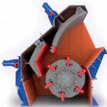
Cut through the big primary crusher ODH with two crushing plates
