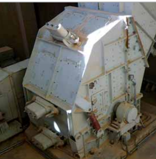
Crusher ODH 1623-13 – limestone crushing 700t/h
