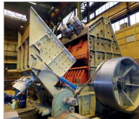
Crusher ODH 2530-13 – limestone crushing 1400t/h
