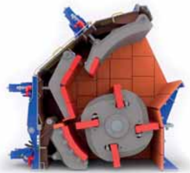
Cut through the primary crusher ODH with three crushing plates
