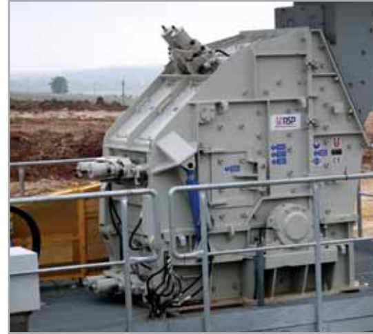
Crusher ODH 1110-23 – limestone crushing 120t/h
