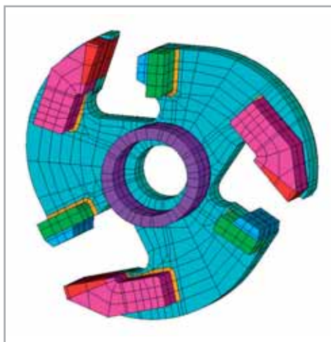
Stress analysis of a crusher rotor disc
