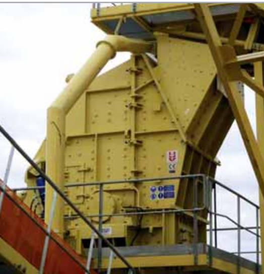
Crusher ODH 1616-22 – limestone crushing 500t/h
