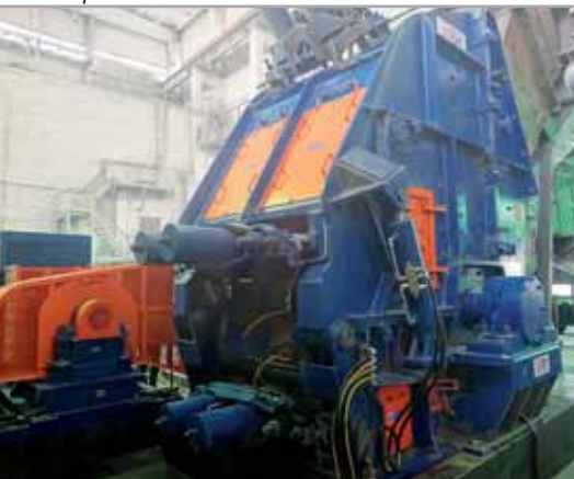
Crusher ODH 1616-23 – serpentine crushing 300t/h
