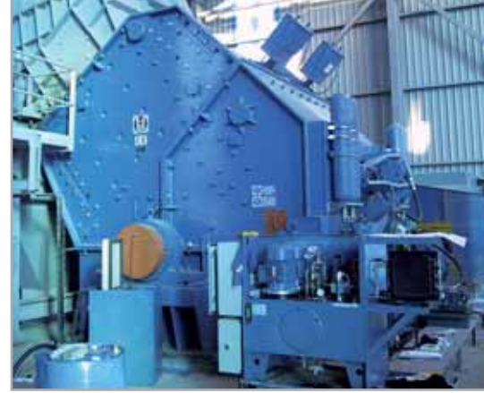
Crusher ODH 2030-13 – limestone crushing 1000t/h
