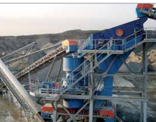
Cone crusher KDC 36 GP – basalt crushing
