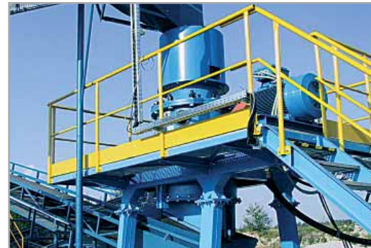
Cone crusher KDC 32 SP – mined gravel crushing
