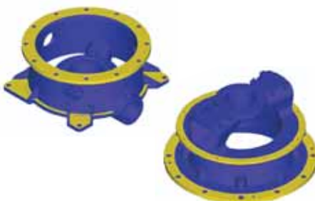
3D model of a crusher KDC stand and body. Control computer display
