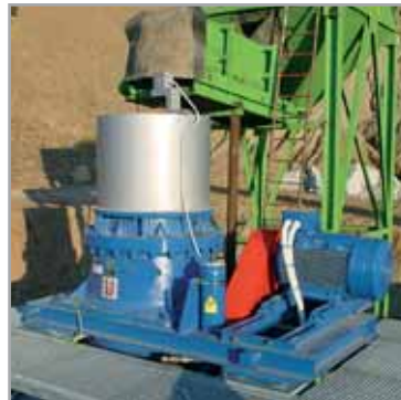
Cone crusher KDC 33 FP – granite crushing
