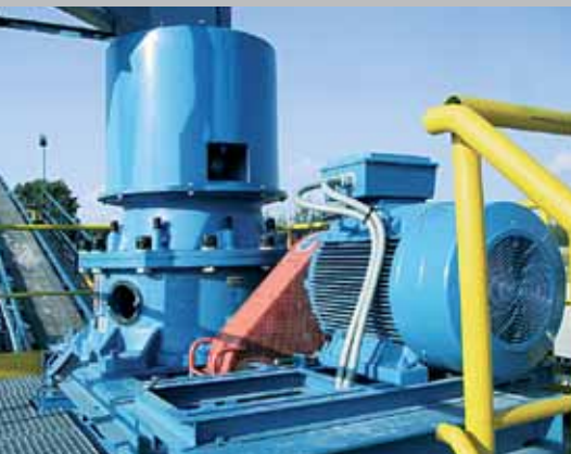
Cone crusher KDC 32 FP—gravel crushing
