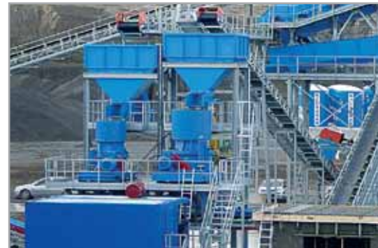
Cone crushers KDC 35 FP and KDC 23 HP – greywacke crushing
