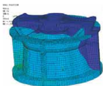
Computing analysis of a cone crusher KDC. Displacements in the solid model
