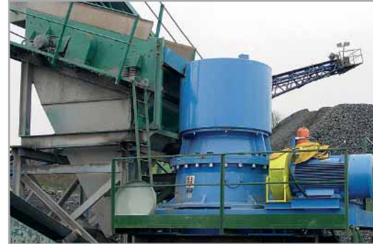
Cone crusher KDC 35 GP – andesite crushing
