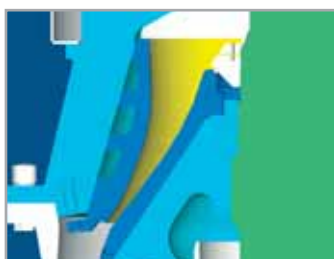
Crushing chamber of the tertiary crusher
