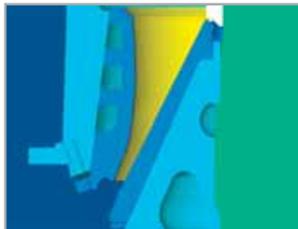
Crushing chamber of the secondary crusher
