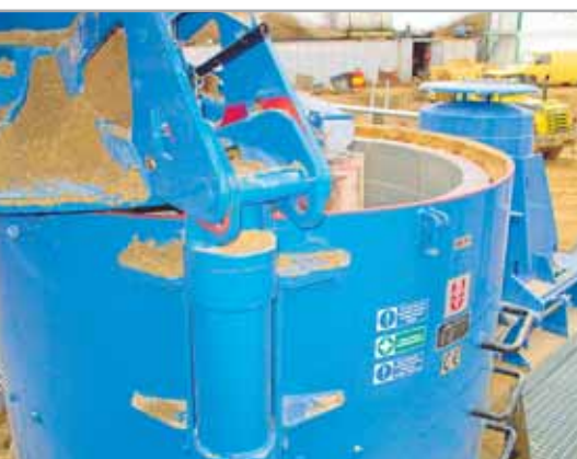
Vertical shaft impactor ODV 1186M – gravel crushing
