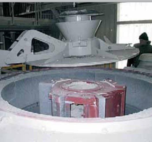
Vertical shaft impactor ODV 1186SM – gravel crushing
