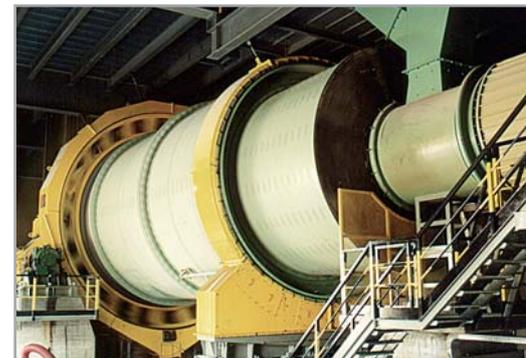
Raw mill  $\varnothing$  5.4 x 11 m with a pre-drying chamber
