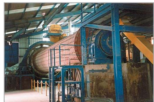
*Examples of cement mills seated on trunnion bearings.*
