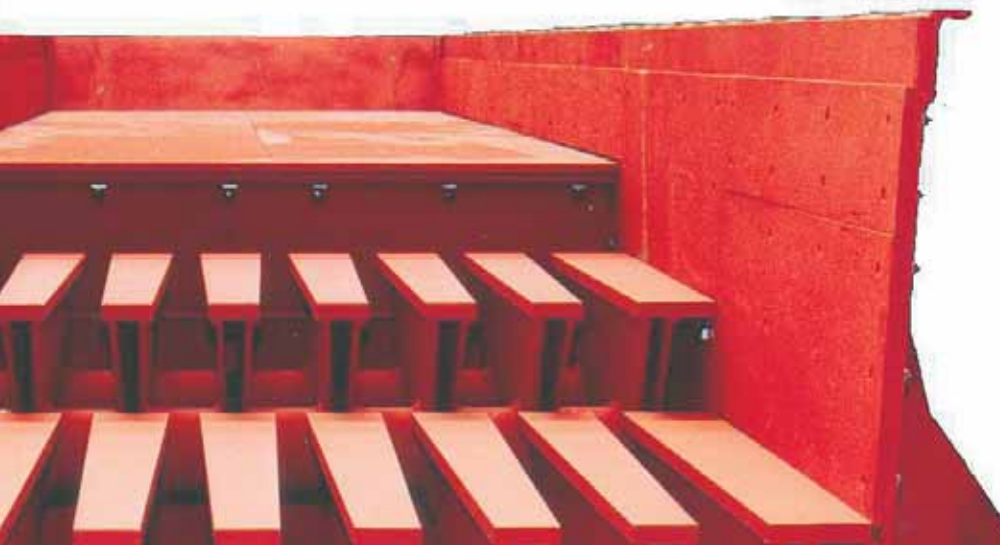
Feeder PVR 1550 x 6000 in the test room in the manufacturing plant
