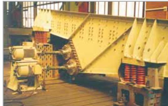
Feeder PVR 1550 x 6000 in the test room in the manufacturing plant
