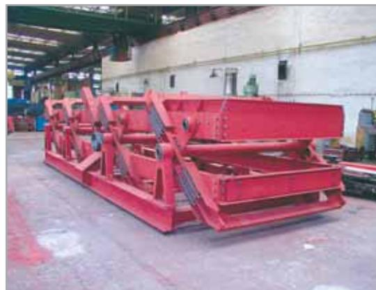
Resonant screen RT 2087/2 – in the manufacturing plant
