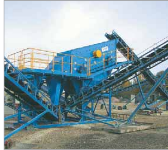
Vibrating screen KDT 2050/2 – granite screening
