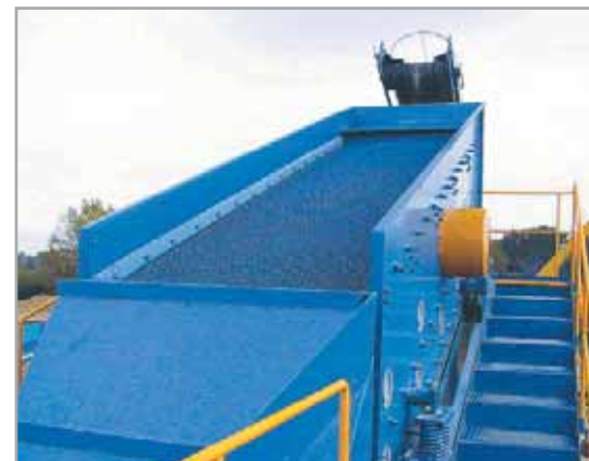
Vibrating screen KDT 1650/3 – gravel sand screening
