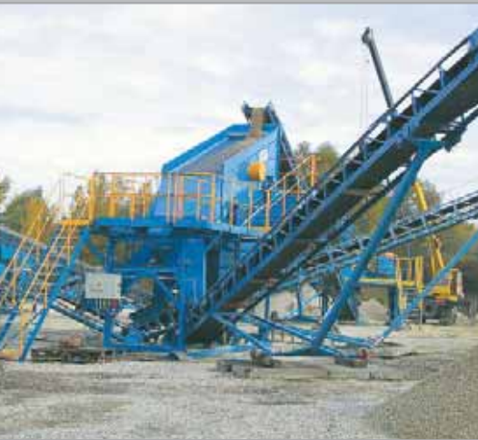
Vibrating screen KDT 1650/3 – gravel sand screening
