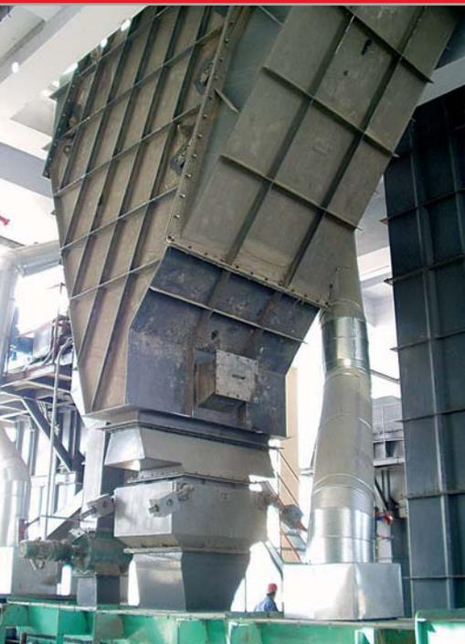
Above: Cascade air separator KVT 1800 as part of the 120 tph cement grinding plant at Qilianhan Cement, China. The photo shows the lower part of the separator with the coarse fraction discharge
