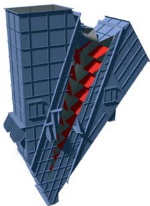
Above and below: 3D models of the cascade air separator KVT
