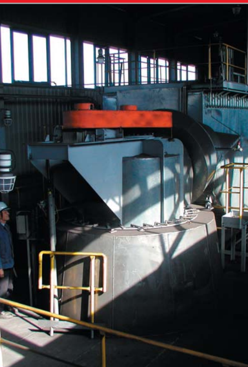
Air separator LTR-R 1650 at a coke grinding plant with 12.5t/h capacity – OKD Ostrava, Czech Republic
