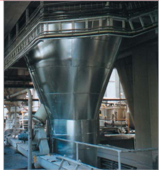
Air separator LTR-R 2500 for 105t/h at the cement raw material grinding plant – Rezola, Arrigoriaga, Spain
